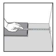
At the end of the first row, put a distance 5-10 mm, to the wall and measure the length of the last plank to be fit
