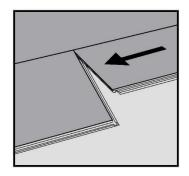
Second plank, second row. Place the plank **gently and tight** to the short end of the previous plank.
