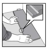
First plank, first row: Place a 5-6 mm thick spacer to the left and position the plank against the wall.
