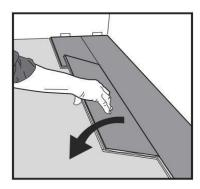
Fold the plank down in a single action movement with a slight press to the left to the short end of the previous plank. During the fold down, make sure the planks are tight against each other.
