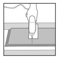
Cut with a jig saw, hand saw, knife or laminate cutter.
