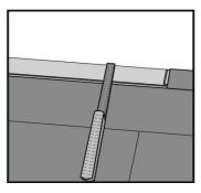
Last row (and perhaps also first row). Minimum plank width should be at least 5 cm. Remember to allow for a gap of 5-6 mm to wall. **Tip!** Put a spacer before measuring Cut the plank lengthwise and glue the short ends.
