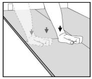
Press or knock slightly along the short end of the installed plank until a click is heard. Do not force or use mallet on seam.
