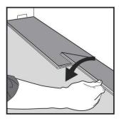
Fold the plank down in a single action movement. During the fold down, make sure the planks are tight against each other. Afterwards press or slightly knock at the short end just installed.
